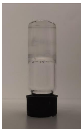
Figure 1. Funori gel – made with Funori 1% w/w and BaCl 2 0.2 M – Tube inversion test
